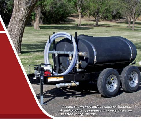
Built for on-site fire protection, the 550-gallon Fire Control Trailer delivers dependable performance when seconds count. Designed for ranches, cotton gins, and remote locations, it comes equipped with a black algae-resistant tank, powerful pump system, fire hose, and galvanized spray equipment. Whether you're battling grass fires or maintaining readiness with stored water, this trailer is your first line of defense.
