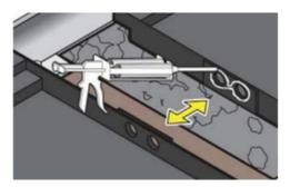
For side pans, make complete circles around the drilled hole on both the first and second pan:
