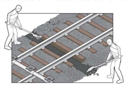
2. The edge of the center drain should be placed at 27.5" from the web of the rail. Insure that the manifold is level witht the rail ties. 1" boards should be clamped to the drain to prevent movement when the void under and around the pipe is backfilled.
