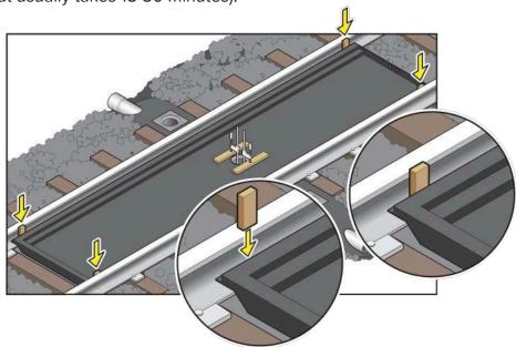
IMPORTANT: <u>BEGINNING WITH THE SECOND PAN</u>, GLUING THE CENTER TRACK PAN TO THE MANIFOLD AND GLUING THE CENTER TRACK PAN TO THE NEXT CENTER TRACK PAN IN THE SYSTEM MUST BE DONE <u>CONCURRENTLY</u> TO INSURE PROPER PLACEMENT.
