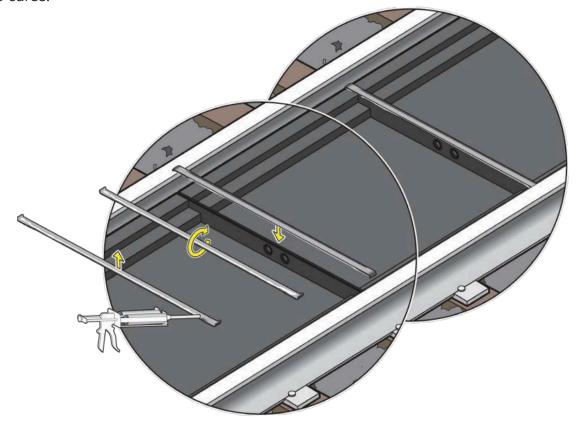
3. If using grates as a walking surface for the Ultra-Track Pans, Composite Model, prepare ten grates for each center pan by inserting two grating pedestals into the diamond on the underside of each grate. These pedestals will prevent the grates from sagging over time.
