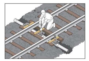
3. Backfill the void with "crush and run" sand. If possible, have additional personnel stand on the boards as added support to prevent the manifolds from moving. Pour sand around the manifold until it is just below the top of the tie. It should very gently be tapped into place to make sure it settles nicely under and around the manifold. Avoid getting sand into the drain.
