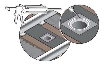
6. Carefully place center pan making sure to line up the drain with the hole in the pan. Re-insert spacers and clamp the pan to the drain. Allow adhesive to completely dry (drying time is dependent on temperature but usually takes 15-30 minutes).
