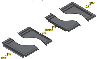
2. It is important to install the center track pans so that they are centered between the two rails. This will facilitate the installation of the center track pan gaskets at the end of this process. In order to keep them centered UltraTech recommends cutting four blocks of quarterboard (5/4) wood 6 inches long. These blocks are to be used as spacers to keep the center track pans centered between the two rails while assembling.
