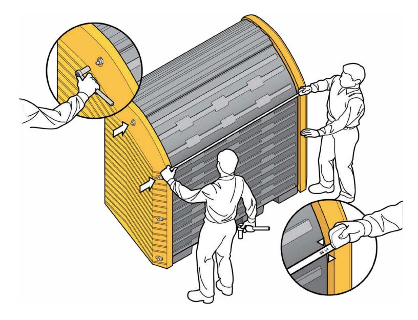
Install the left (5) and right (6) doors by aligning the hinge hole in the door with the hinge hole in the sidewall.
