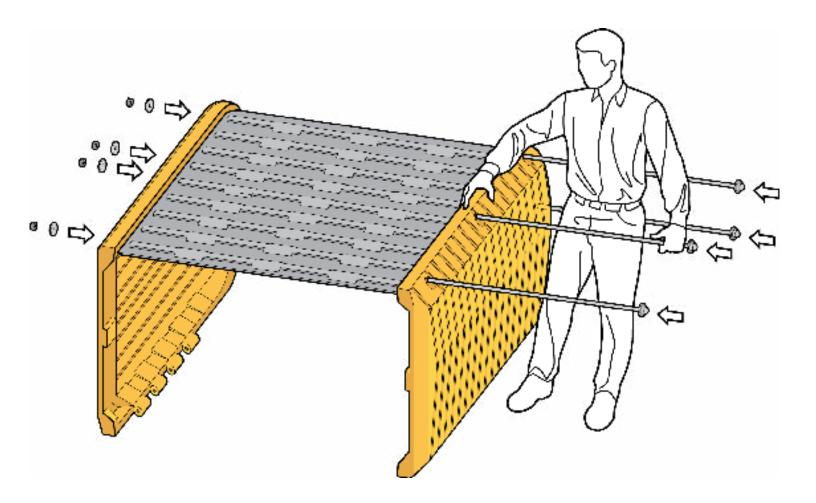
Stand the assembled sidewall and back panel upright and place the all thread rod through the 3rd hole from the bottom using the same steps to attach this rod as the previous rods.
