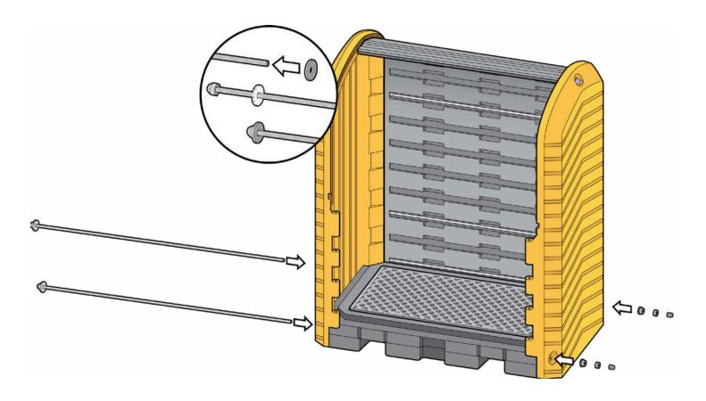
Using a 5/8" socket or wrench hold the acorn nut while turning the nylon locking nut with a 9/16" deep well socket or wrench, tighten the bottom rear attachment rod till both sidewalls are tight against the spill pallet sides.
