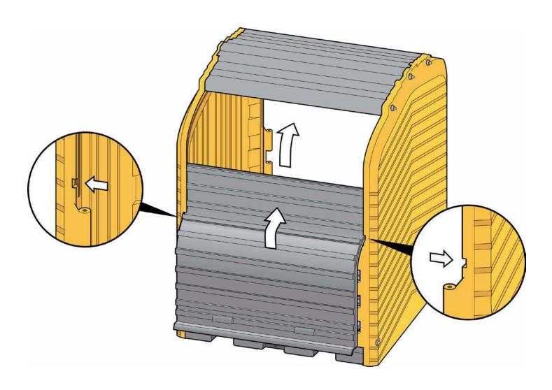
**Step 9** Align the right door (4) hinge with the mating hinge on the sidewall. Align the door hinge pin holes with the hinge pin holes in the sidewall. Slide the hinge pin tube (7) into the aligned holes (Note: It may be necessary to move the door and tap the hinge pin tube with a hammer until the hinge pin tube is fully seated all the way through the hinge holes.) Repeat this step for the remaining right door (4) and to the remaining left doors (5).
