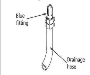
4. Attach the hose assembly (blue fitting and 3/4" drainage hose) to the clear drain fitting on the unit.
