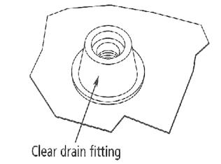
2. From the bottom side of the unit, insert a finger into the center of the clear drain fitting. Pull outward on the inside of the fitting to reveal the external threads.
